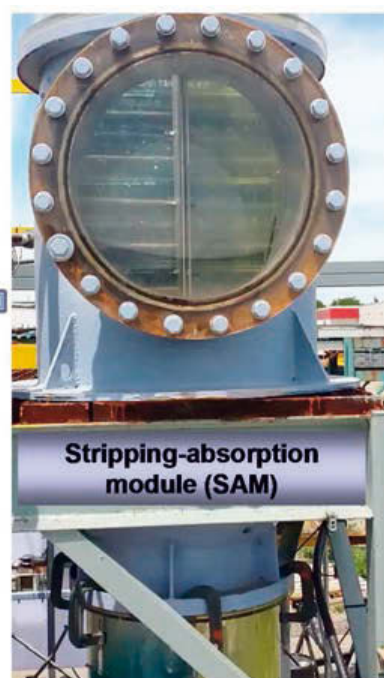
Fig 4: Pass-through distillation pilot-scale unit (left) in operation at Fielding Chemical Technologies, where the stripping-absorption module built by Drystill (right) plays a central role
