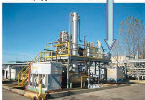
Fig 4: Pass-through distillation pilot-scale unit (left) in operation at Fielding Chemical Technologies, where the stripping-absorption module built by Drystill (right) plays a central role
